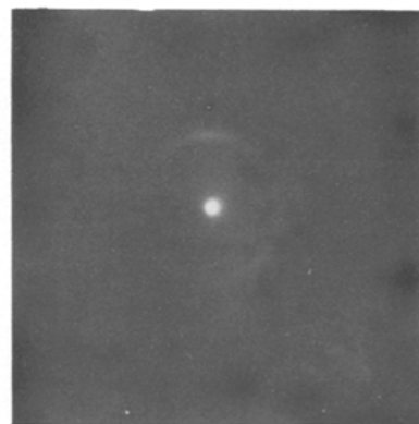
Figure 4 A typical transmission electron micrograph of an amorphous \text{Ni}_{55}\text{Pd}_{35}\text{P}_{10} alloy (bright-field) and the corresponding diffraction pattern.
